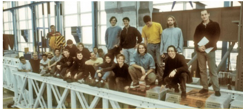
Figure 1. Pontresina Bridge, December 1997: Construction team (students of architecture and TK) on top of 4 kN/m 2 brick loaded adhesively bonded span (without back-up bolts).
