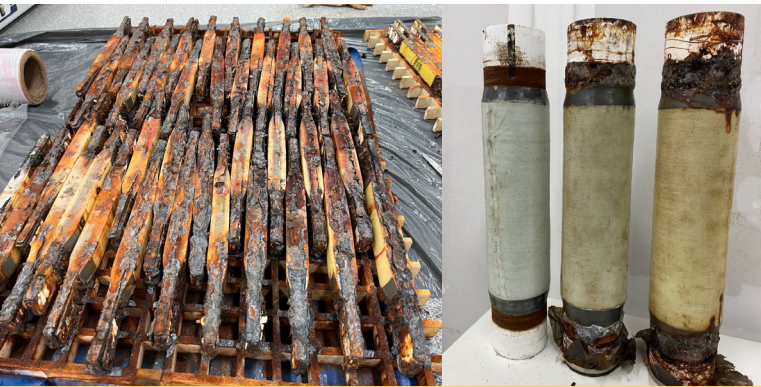
Figure 7. Aged FRP-steel joints and unaged and aged pipes at 55 and 70 °C.
