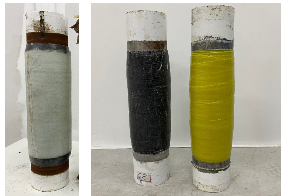
Figure 3. FRP-repaired steel pipe specimens before aging.
