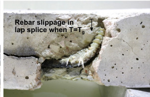
Figure 7. Failure of slab with 90° bent-end lap splices after 75 min of fire exposure, due to slippage of overlapped bars.
