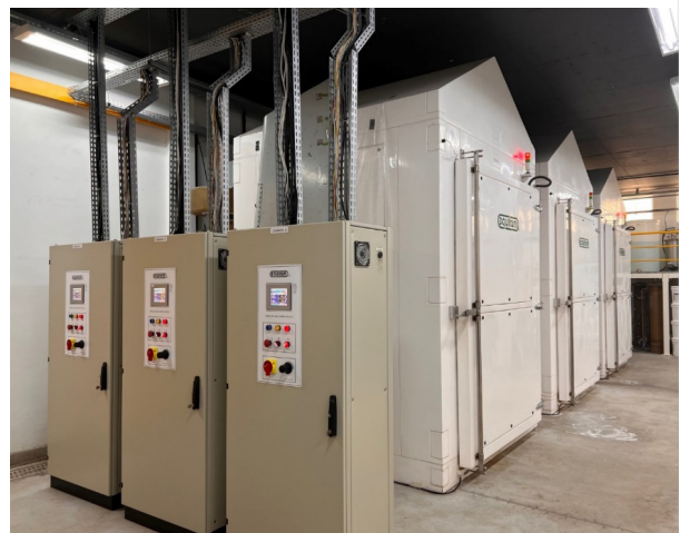
Figure 4. Overview of walk-in salt-spray chambers.
