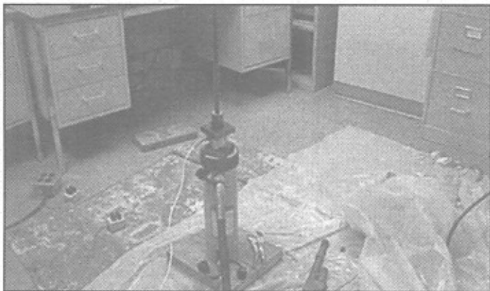
Figure 16. Rapid load testing of CFRP strengthened RC slab.
