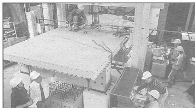
Figure 14. Full-scale testing of deck slab reinforced by leadline bars.
