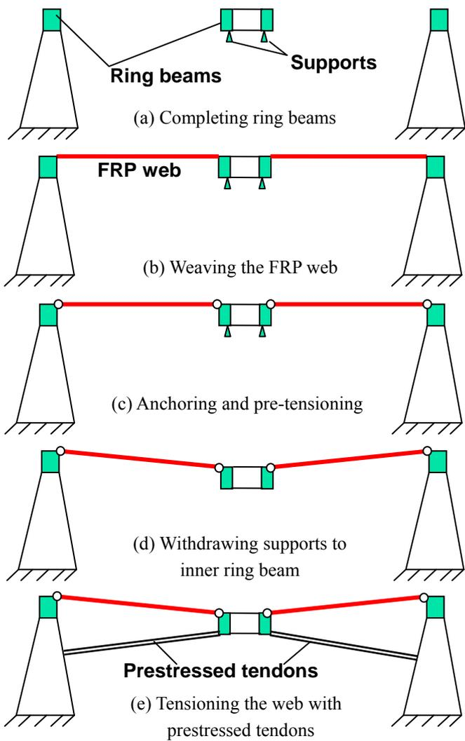
Figure 4. Construction steps
