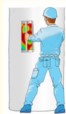
**Figure 2. Concept of Real-Time and Hand-Held Microwave NDE Device**
