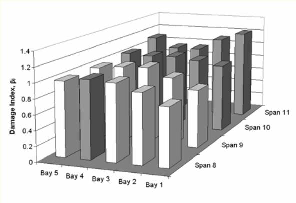
**Figure 8. Damage Indices 20 months after Rehabilitation**
