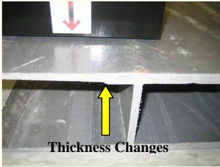
**Figure 7. Detection of Thickness Change in FRP Structural Member**
