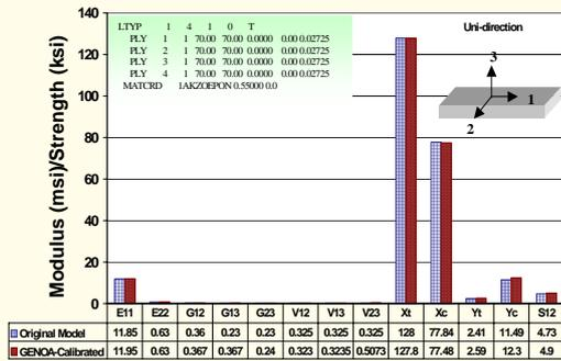
**Figure 4. A Comparison between Calibrated and Original Mechanical Properties of 5HS Laminates**
