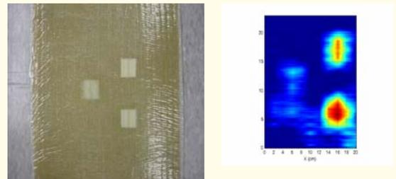
**Figure 6(b). Real-Time Image of a Scanned Area on Multilayered Composites. Depths of Defects and Top, Bottom and Left are 1.0 mm, 1.5 mm and 0.5 mm, Respectively**
