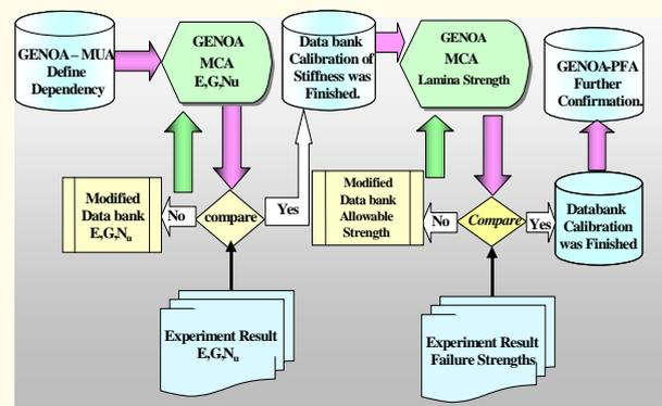
**Figure 1. The Genoa Calibration Procedure**
