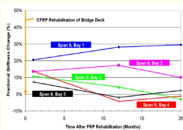
Figure 10. Stiffness Changes in Span 9 After Rehabilitation
