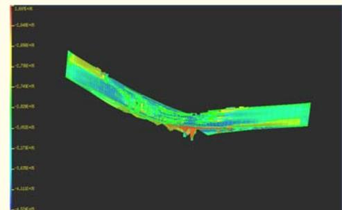
**Figure 12. Ultimate Failure of the Composite Bridge Treadway**
