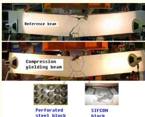
**Figure 1. Comparison of Beams**
