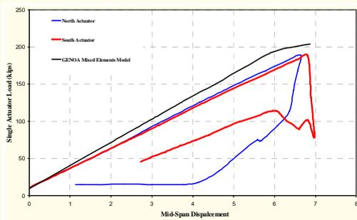
**Figure 13. Comparison between Full-Scale Experimental and GENOA Predicted Results for Load Case 2 (Max Moment)**
