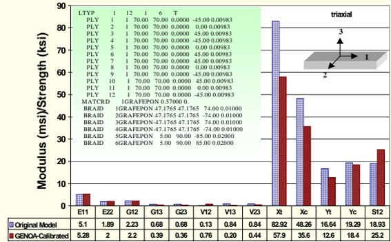
**Figure 6. A Comparison between Calibrated and Original Mechanical Properties of the Triaxial Laminates**
