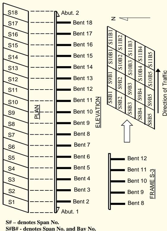
Figure 1. Overview of Watson Wash Bridge and Frame S-3
