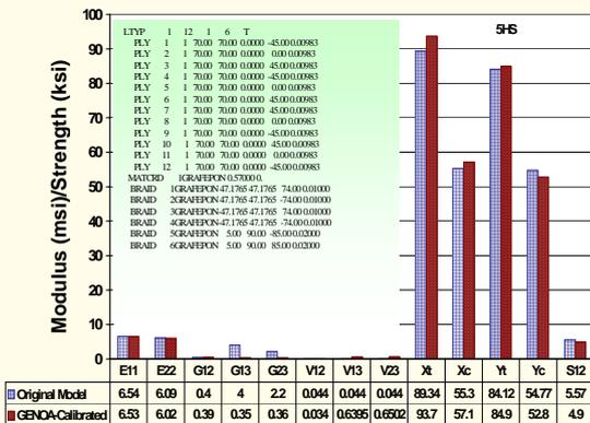
**Figure 5. A Comparison between Calibrated and Original Mechanical Properties of the ±45° Biaxial Laminates**
