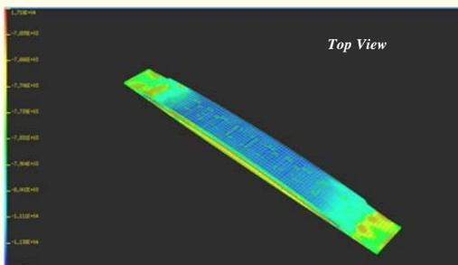
**Figure 14. Generalized Normal Stress  $N_x$  (lb-in) Distribution after 128,140 Cycles (Fatigue Life) – Top View**
