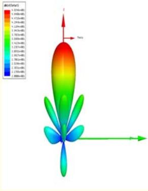
**Figure 3. Microwave Beam of Array Antennae**
