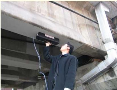
Figure 11(a). Inspection of FRP-Wrapped Girders
