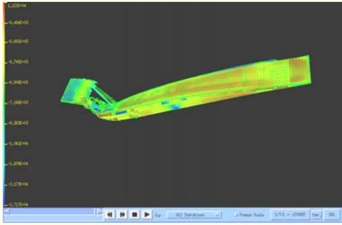
**Figure 8. Generalized  $N_{xy}$  (lb-in) Shear Stress Distribution at the Ultimate Load [280 kips (1,245.44 kN)]**
