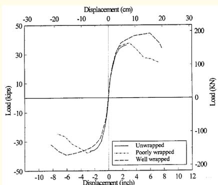
**Figure 1. Debonds and Performance Degradation**
