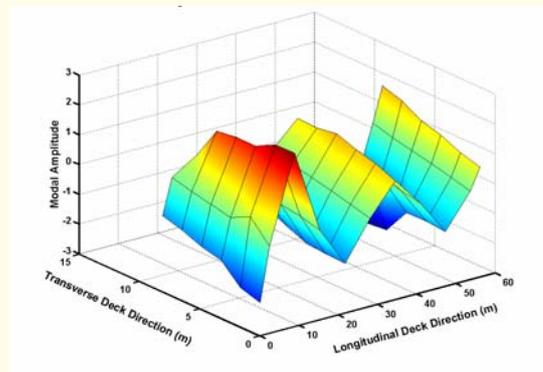
**Figure 5. First Bending Mode, 12 months After Rehabilitation**
