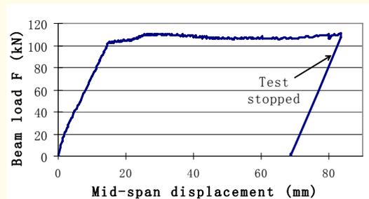
**Figure 2. Result of Compression Yielding Beam Test**
