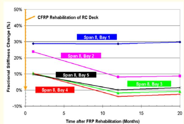
**Figure 9. Stiffness Changes in Span 8 After Rehabilitation**
