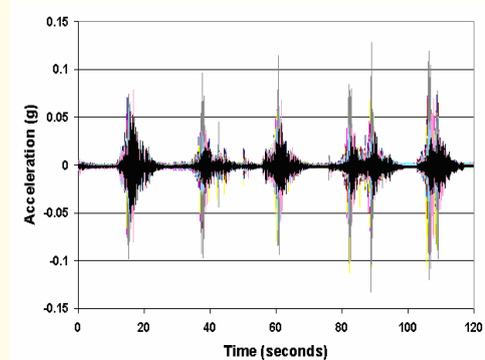
**Figure 4. Typical Measured Acceleration Time History Data**
