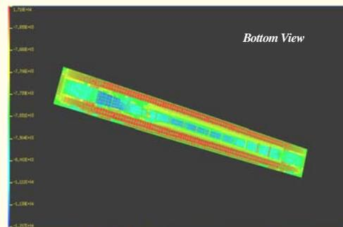
**Figure 15. Generalized Normal Stress  $N_x$  (lb-in) Distribution after 128,140 Cycles (Fatigue Life) – Bottom View**
