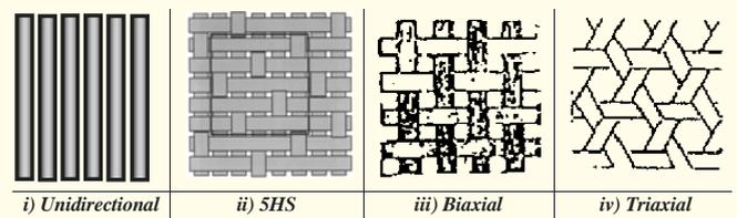
**Figure 2. Types and Geometry of Fibers Used in the FEM Analysis**
