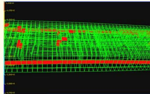
**Figure 11. Zoom-In Top View of Damage Distribution Just before the Ultimate Failure**
