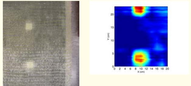
**Figure 6(a). Real-Time Image of a Scanned Area on FRP-Wrapped Concrete. The Top Defect is at 1.5 mm Depth and the Bottom Defect is at 1.0 mm Depth**
