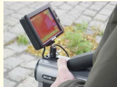
**Figure 10(b). Thermography Using Infrared Camera**
