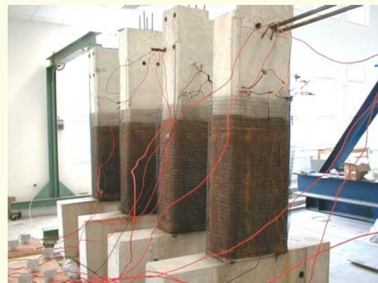
Fig. 1: Accelerated corrosion of RC columns.
