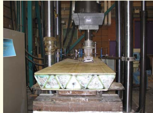
Fig 3: Test Setup of Shear-Keyed Deck Module
