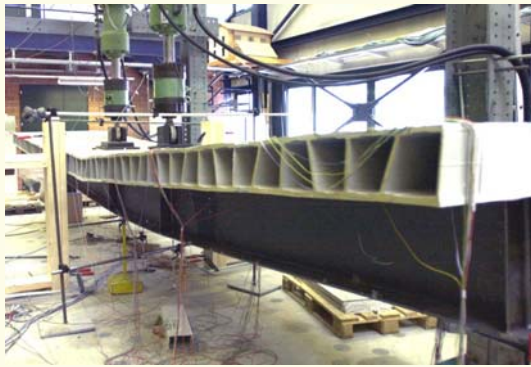
Fig. 4: DuraSpan system adhesively bonded to steel girders (test girders at onset of failure)
