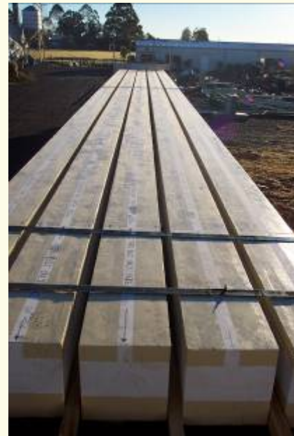
Fig. 6: 20m Long Hybrid Beams Ready to be Shipped to Site
