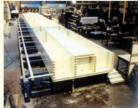
Fig. 1: GFRP box beam in construction using ACCS planks
