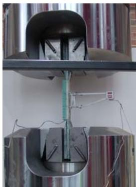
*Figure 3: Setup for Tension Test*
