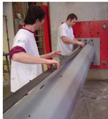
*Figure 5: Application of the High Modulus FRP Strips to the Monopole*
