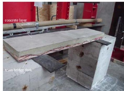
Figure 9: GFRP Truss Bridge Deck with Concrete Layer
