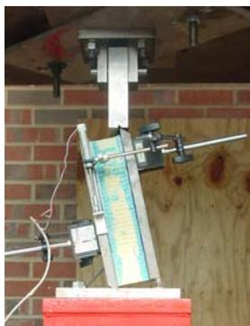
*Figure 2: Setup for Shear Test*
