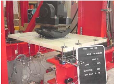
*Figure 1: Test Setup for FRP Sandwich Panels Using a Concentrated Tuck Tire Loading at Mid-Span*
