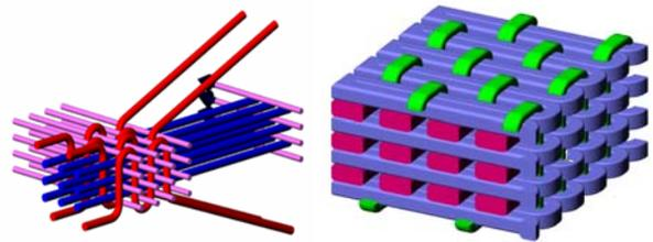
Figure 8: Weaving Process and Resulting Fiber Architecture
