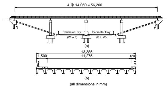
Figure 1 – Schematics of PTH 9 Overpass
