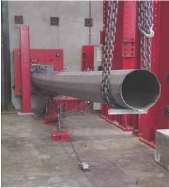
Figure 6: Strengthened Monopole Near its Ultimate Capacity
