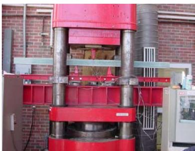
*Figure 4: Setup for Flexural Test*
