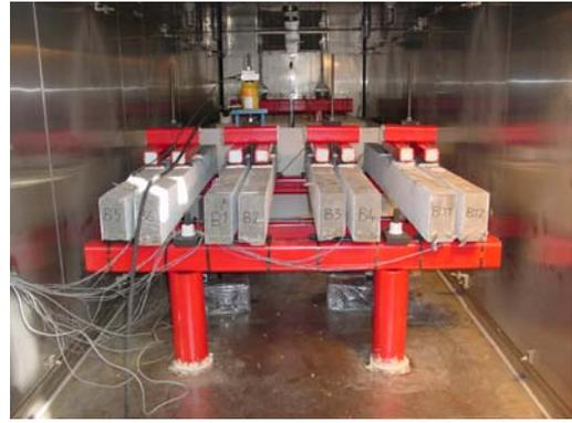
*Figure 10: Beams in the Environmental Chamber*
