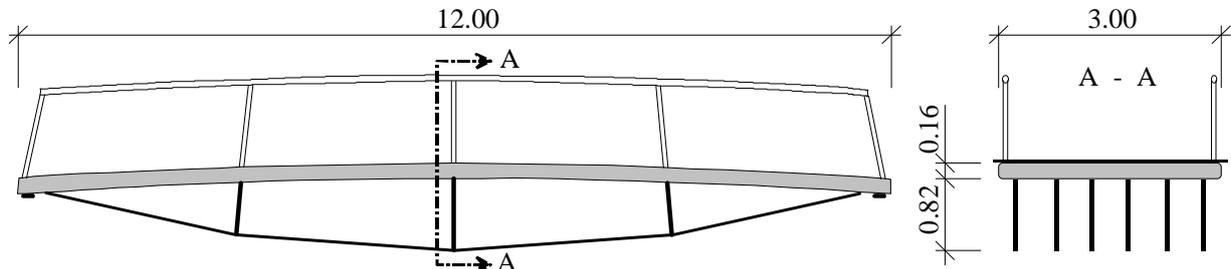
Figure 1: Geometry and main dimensions of the bowstring arch bridge. All measurements are in [m]
