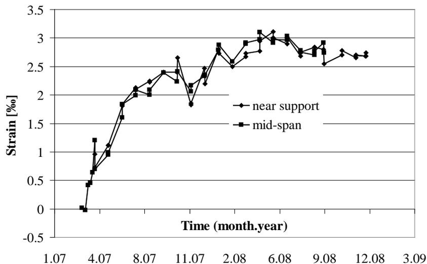
Figure 13. Results of strain measurements from 2007 until 2009 lateral to the glulam deck
