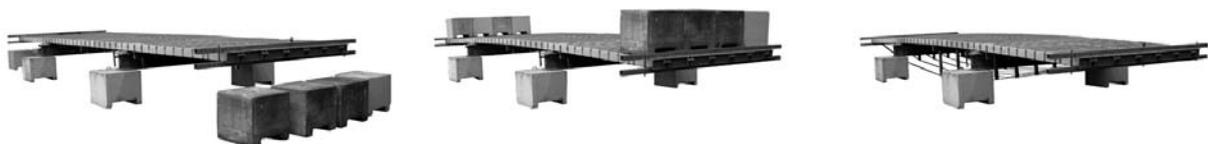
Figure 5. “Drawing of the bow”: Left: Flat glulam deck supported at quarter-points. Center: Bow shape of deck achieved by loading the cantilever ends. Right: Struts and cables keep the bow shape of the plate after removing the load
