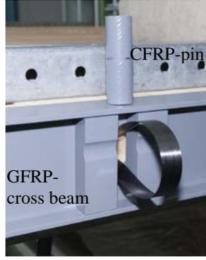
Figure 7. Termination of a pin-loaded CFRP strap before tensioning. The length of a pin is 125, and the diameter 40 mm
