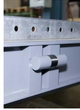
Figure 8. Termination of a pin-loaded CFRP strap after tensioning. The fibre lay-up of the CFRP-pin is  $0/\pm 45^\circ$  (Tenax UTS/EP)
