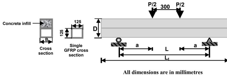
**Figure 1.** Flexural test set-up.
