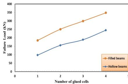
**Figure 3.** Failure load and number of cells relationship
