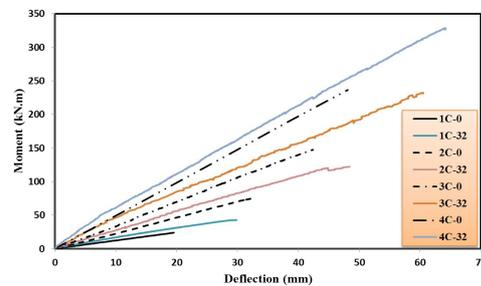
**Figure 4.** Moment-deflection behaviour of hollow and filled beams
