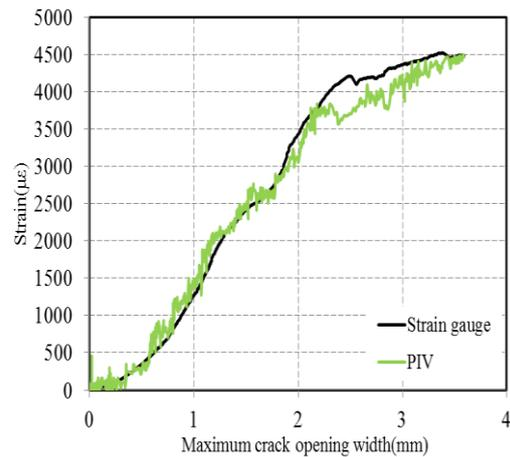
Figure 7 Strain gauge vs. PIV measurement results
