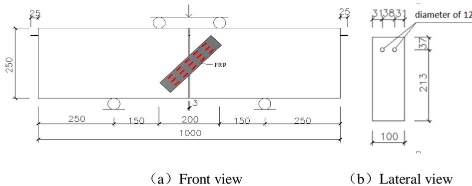
Figure 1 Details of small beam specimens
