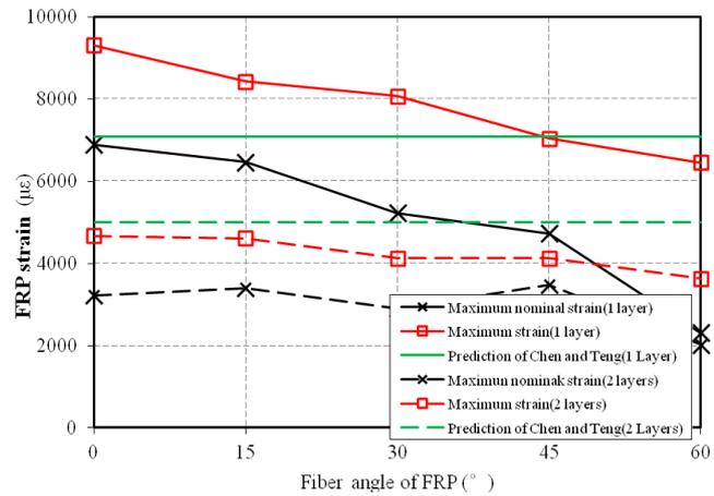
Figure 5 Effect of fiber angle on FRP strain
