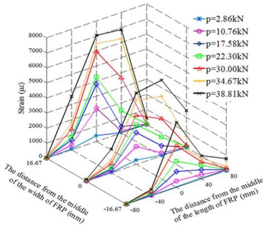
Figure 4 Typical FRP strain distribution
